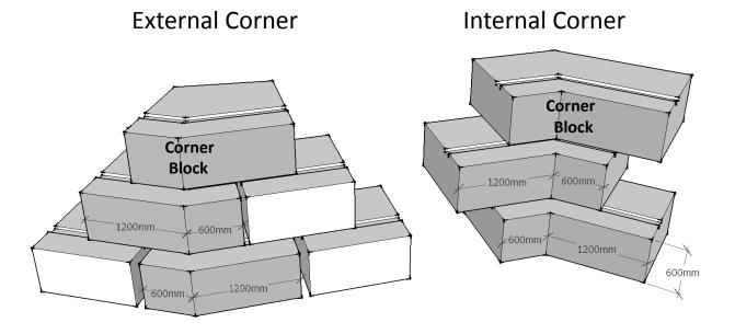
Graviti®Block corners - External & internal are:-
